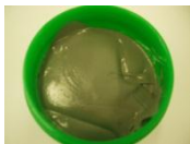
Solder paste immediately after filling no separation
