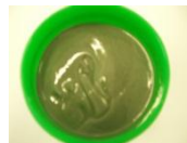
Solder paste after longer storage slight separation
